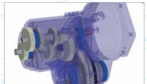
Automotive transaxle model with housing in Finite Elements
