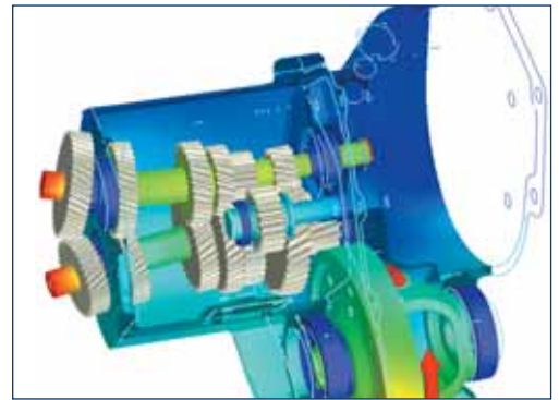
Deflection of flexible housing, shafts and gears
