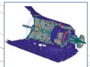
Full dynamic model of an automatic transmission
