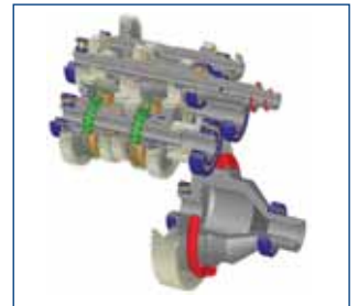
DCT model created by Romax as part of a customer's design project
