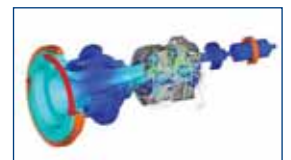
Drivetrain Eigen frequencies
