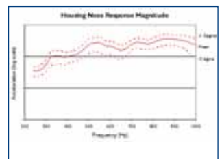
Understanding the effect of manufacturing tolerances on the variation of housing vibration
