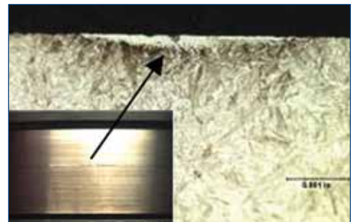
Raceway defect identified from grinding damage
